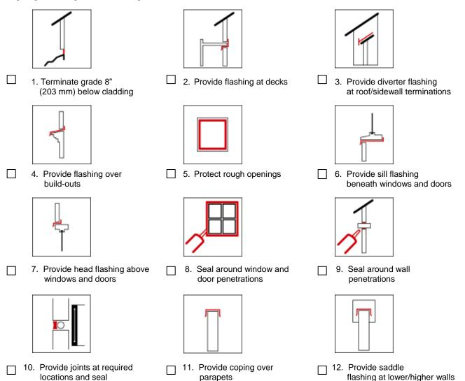
It has been said that, "As much as 90 percent of all water intrusion problems occur within 1 percent of the total building exterior surface area. The 1 percent of the structure's façade contains the terminations and transition detailing that all too frequently lead to envelope failures." <sup>1</sup> By paying close attention to construction details at cladding terminations, water intrusion can be prevented and building durability enhanced.
